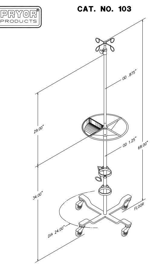
FOUR-LEGGED HEAVYWEIGHT STAINLESS STEEL BASE 24.00" DIA. STAINLESS STEEL BASE POLE WITH, 4 EA SOFT RUBBER 3" BALL BEARING CASTERS, PATIENT SUPPORT WHEEL, WITH UTILITY TRAY. OXYGEN TANK HOLDER, WHICH HOLDS UP TO AN E SIZE CYLINDER. STAINLESS STEEL S HOOK, TELESCOPING STAINLESS STEEL I.V. POLE WITH SLOW DESCENDING INNER POLE. 4 STAINLESS STEEL HOOKS. 99" FULLY EXTENDED 68" COMPRESSED. SHIPPING BOX IS 18 X 18 X 34-3/4 BOX. SHIPPING WEIGHT 32LBS.
