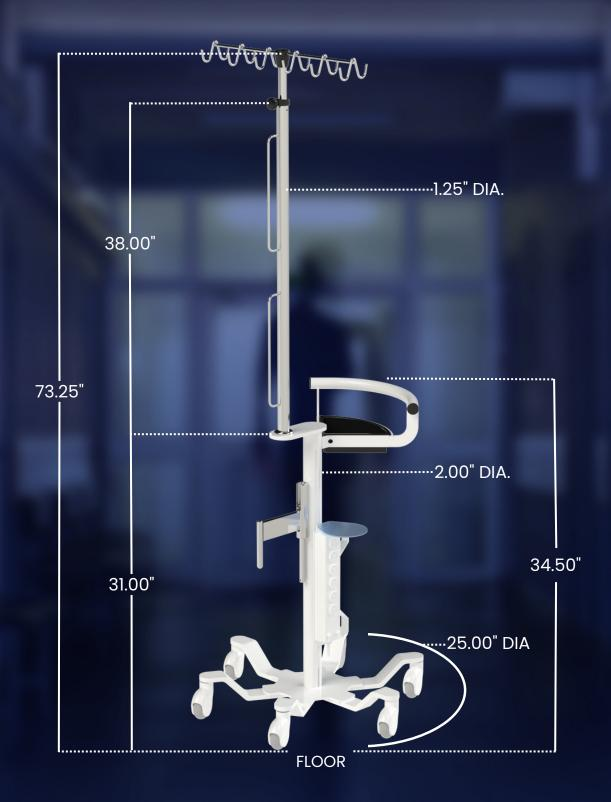
Six-Legged heavyweight base 25.00" Dia. White epoxy finish with, 6 ea. soft rubber 3.00" ball bearing casters. 6-outlet electrical strip, with protective cover and cord wrap. Patient support handle. Off-set stainless steel top pole with slow descending inner pole. Bed transport hitch. 12 stainless steel hooks, 97.00" fully extended, 73.25" compressed. Hex shipping box is 24.00" x 27.00". Shipping weight 59 lbs.
