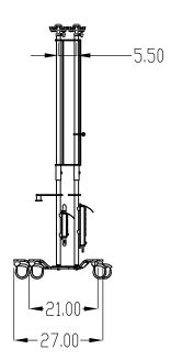
SIX-LEGGED HEAVY WEIGHT BASE 28.00" X 27.00". OFF WHITE EPOXY FINISH. WITH, 6 EA, SOFT RUBBER 3" BALL BEARING CASTERS, 2 EA LOCKING. CORD WRAP WITH 2 EA. 6-OUTLET, 1 EA. 4-OUTLET UL APPROVED HOSPITAL-GRADE ELECTRICAL STRIP, WITH PROTECTIVE COVER. STAINLESS STEEL PUMP ADAPTER WITH STAINLESS STEEL PUMP DEFEAT HANDLES AND SLOW DESCENDING TELESCOPING POLES WITH 18 STAINLESS STEEL HOOKS. 100.00" FULLY EXTENDED 77.00" COMPRESSED. SHIPPING BOX IS TBD SHIPPING WEIGHT IS APPROXIMATELY 107 LBS.
