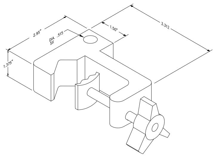
BLACK ANODIZED ALUMINUM CLAMP WITH DETACHABLE KNOB, SELF ADJUSTING THRUST PLATE, CLAMP ADJUSTS FROM 1/2" TO 1-1/2". SHIPPING BOX IS. 12 X 12 X 18. (BULK PACKAGING) SHIPPING WEIGHT IS 45 LBS.
