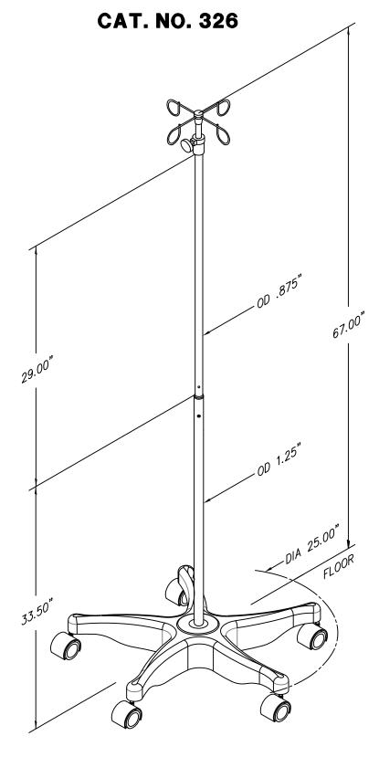
FIVE-LEGGED OFF WHITE EPOXY COATED BASE 25" DIA. WITH 5 EA PLASTIC 2" HOODED CASTERS. STAINLESS STEEL BASE POLE. TELESCOPING STAINLESS STEEL TOP POLE, WITH SLOW DESCENDING INNER POLE. 4 STAINLESS STEEL HOOKS. THE TOP POLE REACHES 94" FULLY EXTENDED 67" COMPRESSED. SHIPPING BOX IS 33.5 X 23.5 X 5.5. SHIPPING WEIGHT 13 LBS.
